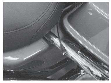
Gerbing Temperature Controller connects to the external Battery Harness here.
